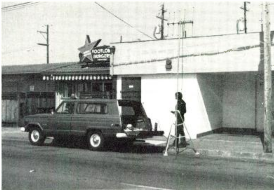
The Scala CA5-150 yagi antenna used as part of KRED/KPDQ's three-hop RPU system.
