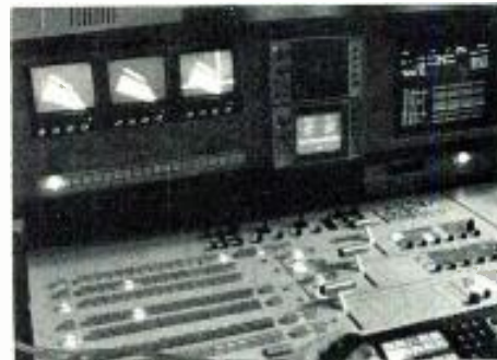
ADO system at The Post Group can be configured for single-channel or multiple-channel operation.
